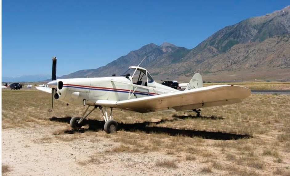
"Worst bent prop I've ever seen." Pawnee damaged by instant violent updraft during the start of a tow at Nephi, Utah. The airport is surrounded by thousands of acres of green farmland - which would not provide any dirt to make a visible "dust devil" out of any strong vertical vortex convection that might be pushed by a cross wind onto the runway. Any surface ± bare rock, pavement, green cropland, whatever ± can produce invisible vertical vortex convection events that can catch pilots and ground crews off guard. Photo by Bob Thompson
