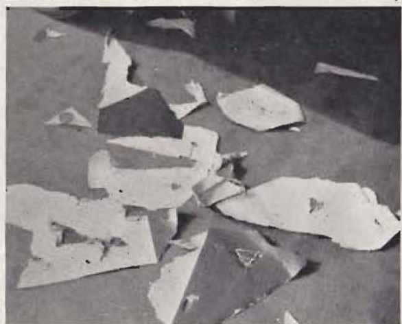
▲ Hailstone damage to Voss's Cobra 15 ▼
